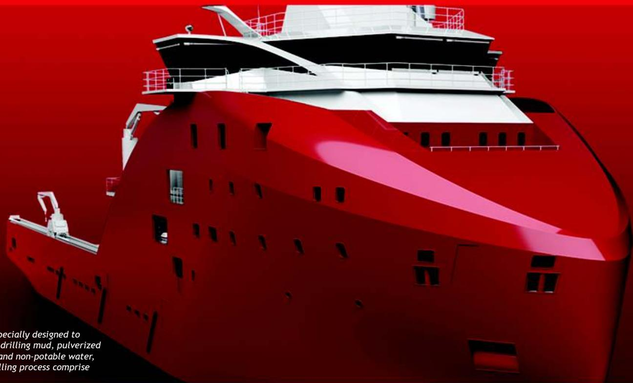
*Platform Supply Vessel ship specially designed to supply offshore oil platforms drilling mud, pulverized cement, diesel fuel, potable and non-potable water, and chemicals used in the drilling process comprise*
