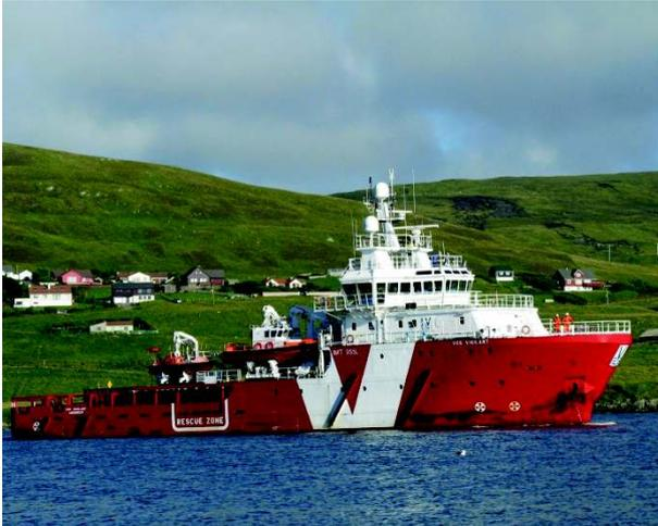
**Purpose** : Used for transportation of dry bulk cargo and also fluids to offshore installation. Can also be used to provide emergency rescue and evacuation support for offshore facilities, rigs and platforms. It also acts as a reserve radio station and provide on scene coordination
