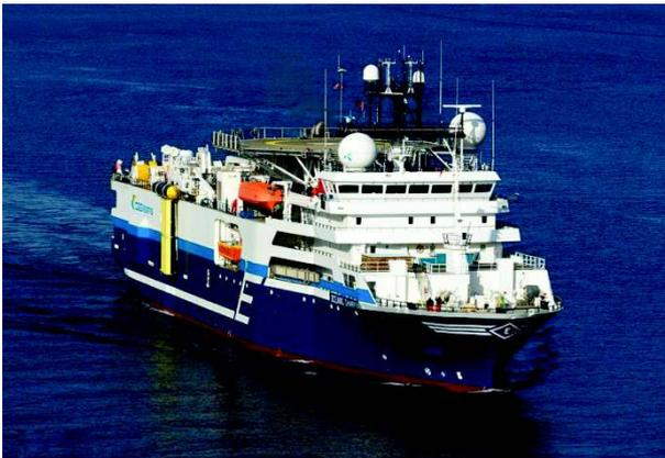
**Purpose** : Used for seismic purposes in the high seas - mainly with the intention of locating hydrocarbon deposits. The equipment onboard is specifically designed to pinpoint the best location to drill for oil.
